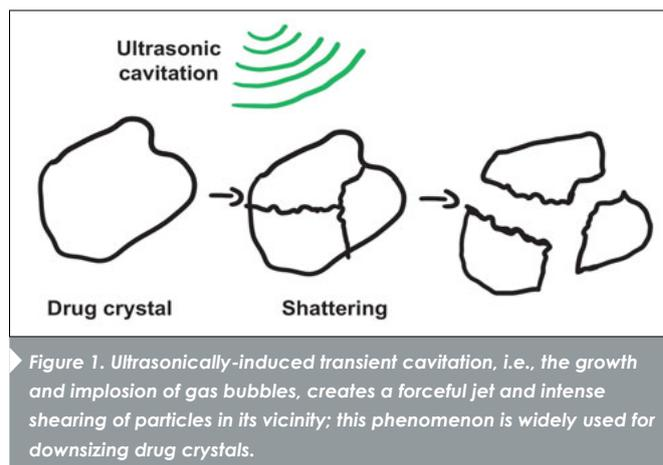
Figure 1. Ultrasonically-induced transient cavitation, i.e., the growth and implosion of gas bubbles, creates a forceful jet and intense shearing of particles in its vicinity; this phenomenon is widely used for downsizing drug crystals.
