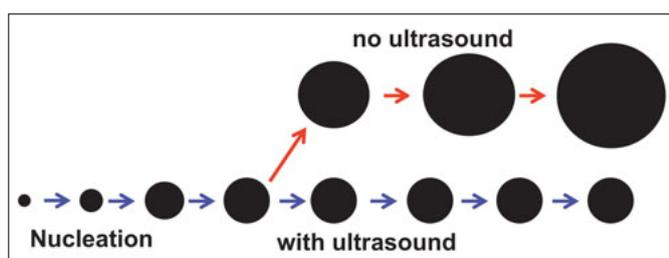
Figure 2. Ultrasound can be used for controlling the growth of crystals in solution by homogeneously dispersing the precipitating material.
